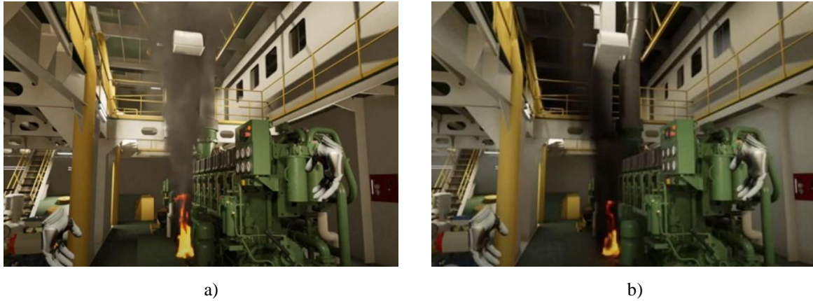
Figure 7. Fire and smoke on the lower deck of the engine room: a) VR generic, b) CFD-based.
